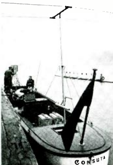
The television-transmitting launch Consuta . Camera control equipment on the launch. Marconi camera on its vibration-free mount.
